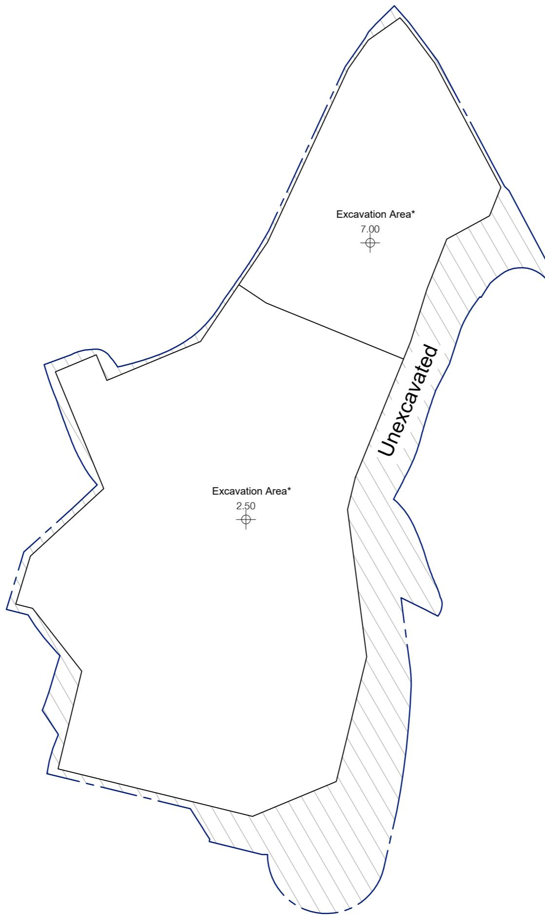
\*The excavation area is about 13,500m<sup>2</sup> and the excavation depth is about 13.5m. The excavation area and depth are subject to future detailed design on foundation based on further geotechnical information.
